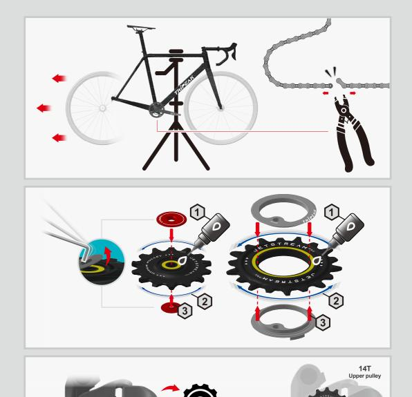
the tool based on the original screw specifications). Replace it with the AOPW upper pulley (ensure the side with the text is facing outward), and gently tighten the existing upper pulley screw.
